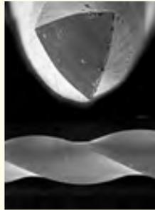
**Figure 2:** SEM images showing the cross-sectional and lateral views of an active file with sharp cutting edges.
