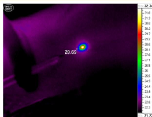
**Figure 2:** The thermogram demonstrates instantaneous heating of only the air at the end of the laser fiberoptic tip with the laser beam Energy 300 mJ.
