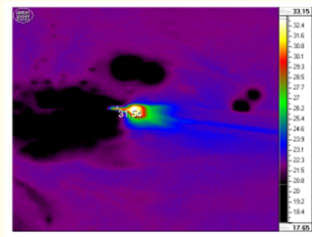
**Figure 1:** The thermogram demonstrates the heating of the ultrasonic needle of the phacoemulsifier at 40% ultrasound power without cooling in a continuous mode.
