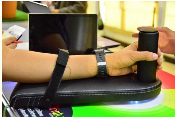
Figure 1: Hand skate or 'Phukphon' designed to control joystick for gameplays.
