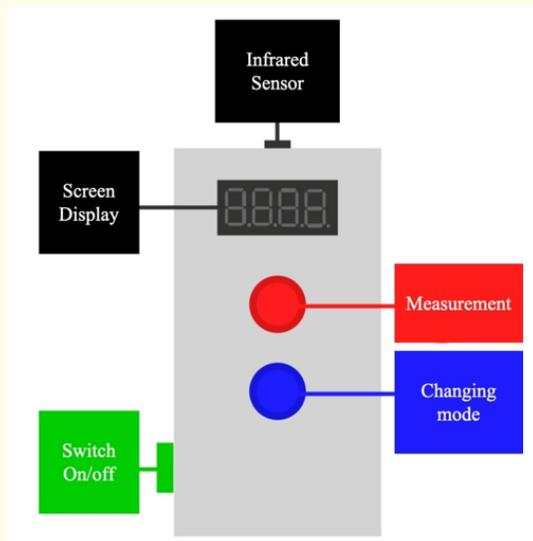
**Figure 3:** Infrared sensor (The inspect).
