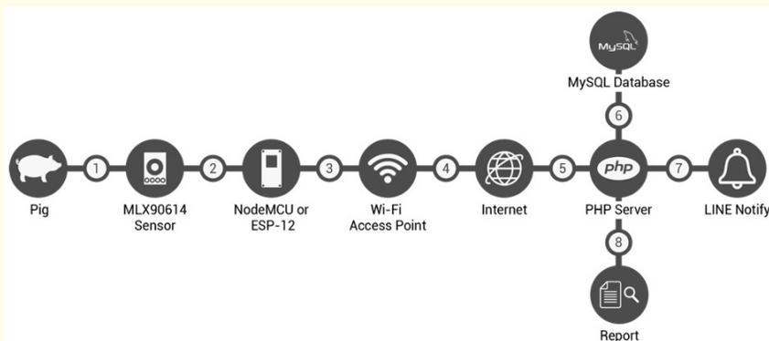
Figure 2: Systemic architecture of the measurement system used to measure the body temperature of sows.
